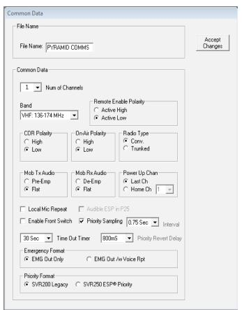
*Tx Audio*: If the mobile Tx audio from the SVR-N300 to the mobile is connected to the mic input, select Flat response. If connected after pre-emphasis, select Pre-Emp.
